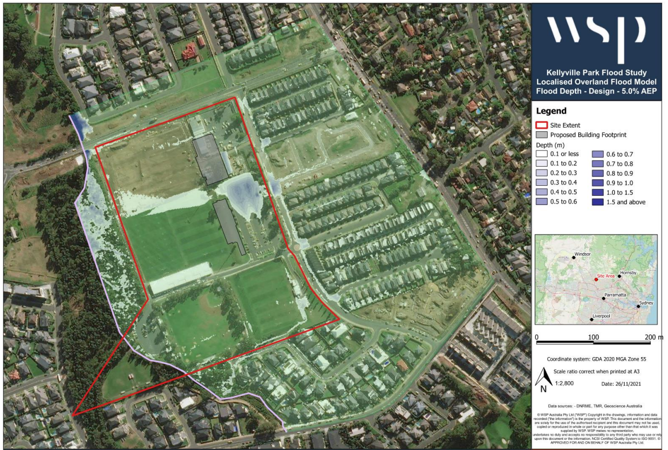
flooding report: Figure 2 - Localised overland flow depth in 5% AEP event (Source: WSP Flood Impact Assessment July 2022)
